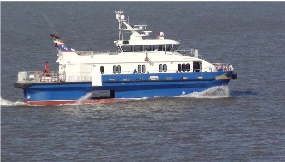
FIGURE 24: WIND TURBINE SERVICE VESSEL. SUCH VESSEL COME IN MANY SHAPES AND SIZES AND ARE MADE FOR VERY DIFFERENT OPERATING CONDITIONS, SUCH AS VERY SHALLOW WATER OR OPEN SEA.
